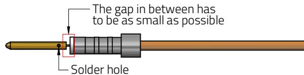
**Step 4.** Push cable with small center contact into connector main body
