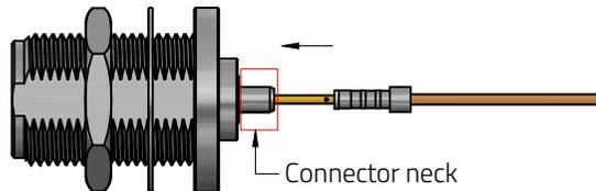
**Step 5.** Crimp ferrule with tool hex size : .1" (check point 4)
