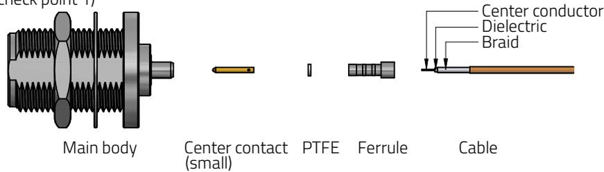
**Step 2.** Pre-tinned cable center conductor (optional, see check point 2)
